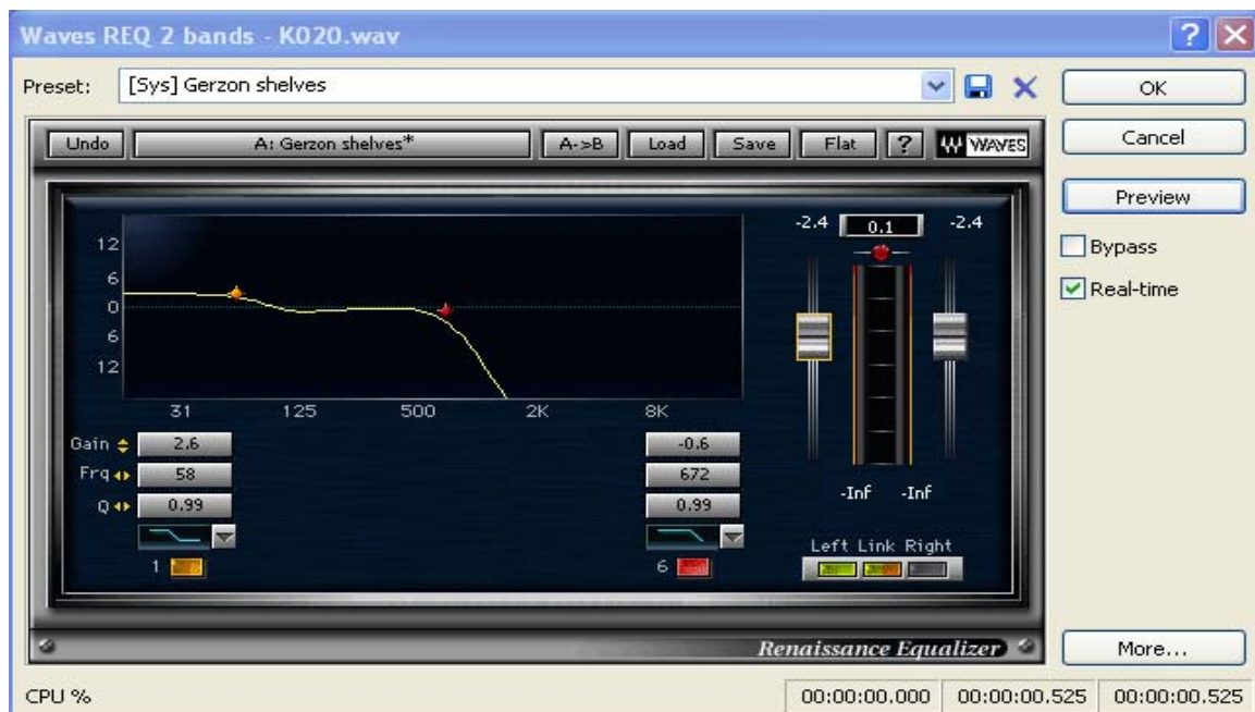
Fig 11.20: 2 Band with low shelf and low pass
